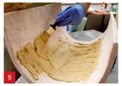
By using Thix A the A1 becomes a gelcoat which can be applied on vertical parts.
