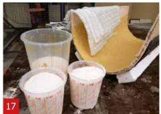
In the meantime weigh 450 g A1 liquid and 900 g A1 powder. Also cut 4 pieces of triaxial fibre (same size as the mould you will be using).
