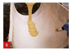
Apply the A1 on the mould and spread with a brush.
