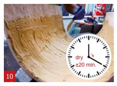
The surface must reach a thickness of 3 mm. Let the panel dry for ± 20 min.
