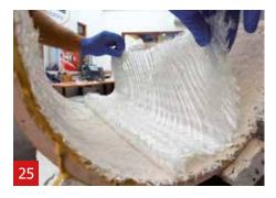
Apply another layer of triaxial fibre. Repeat step 22, 23 and 24 untill you have 4 layers of triaxial fibre. When finished clean the brush with water.
