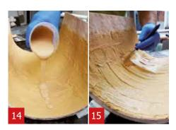
Apply a little amount of A1 on the surface and devide it equally 15. This way you create a smooth finish layer.
