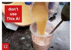
For the 2nd layer of A1 we weigh 125 g A1 liquid, 250 g A1 powder and 250 g yellow sand, and mix them like in step 3 and step 4.
