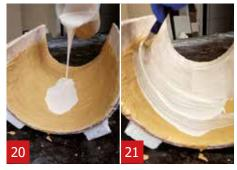
Apply a thin layer of A1 on the surface and devide it equally with a brush 11.
