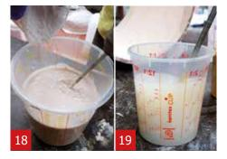
Add the A1 powder slowly to the A1 liquid and stir with the mixer until you have a smooth mixture 18. Clean the mixer directly after use in water 19.
