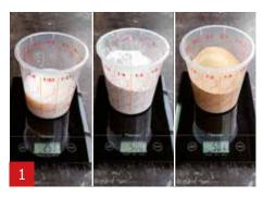
Calibrate the scale and weigh 250 g A1 liquid (1 part), 500 g A1 (2 parts) powder and 500 g yellow sand.
